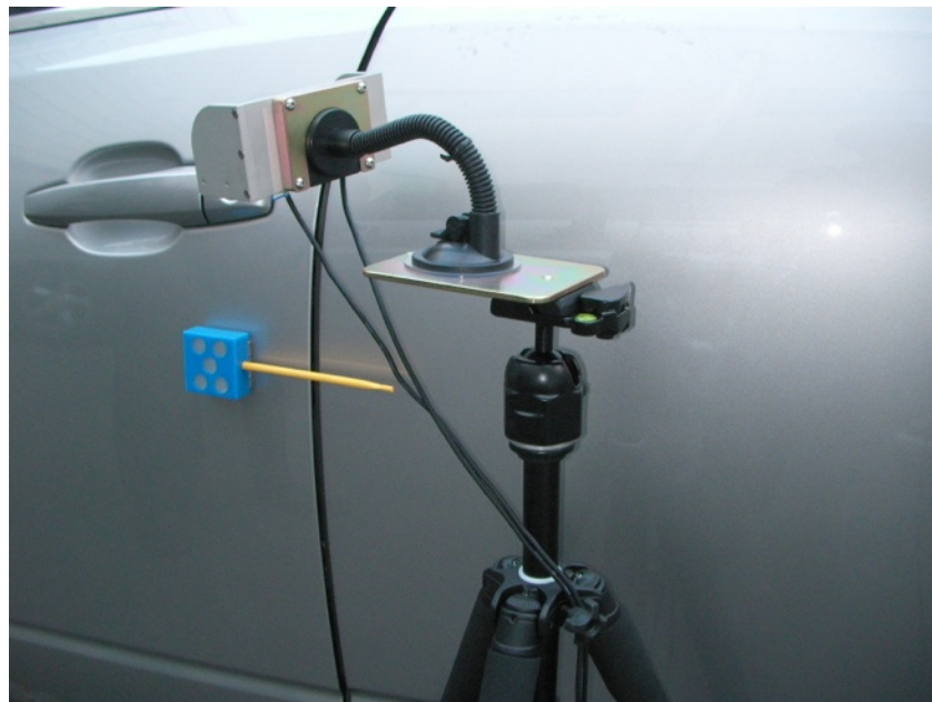
pic9. Measure the speed of a side door
