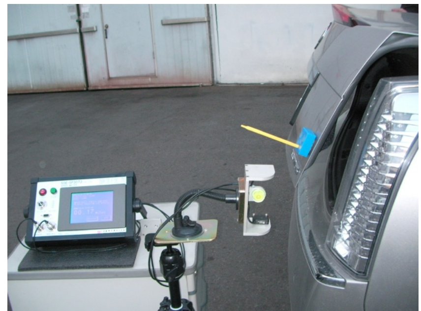
pic10. Measure the speed of a trunk
